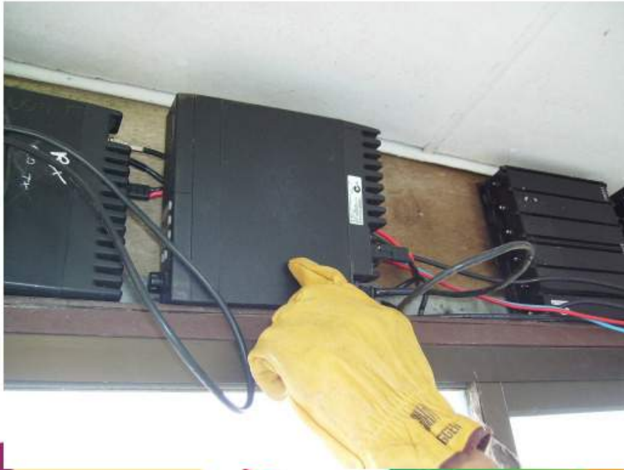
The repeater comprising of 2 Motorola GM300s and diplexor.
